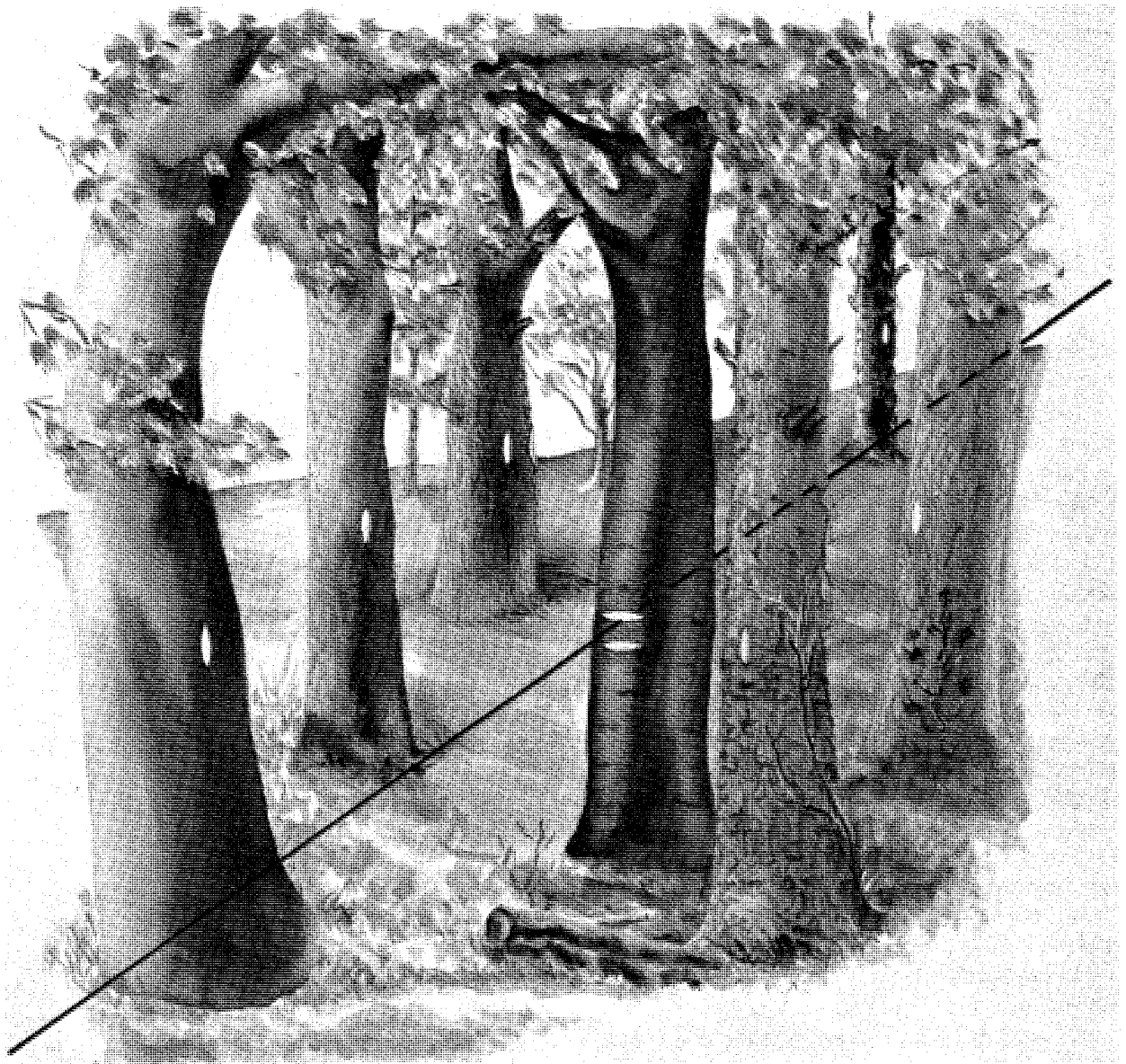
FIGURE 63.—Marking a line through timber.
